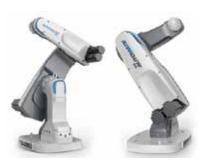
**Latest TAL BRABO** 5 AXIS ROBOT with controller specially for training.
